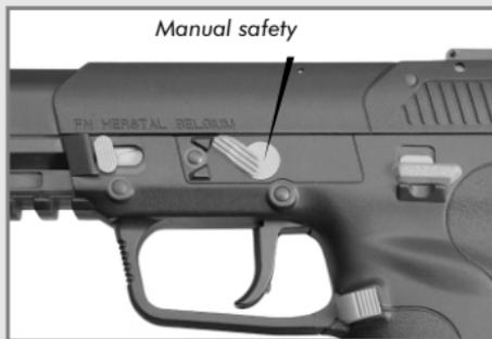
*When the manual safety is at the (raised) 'safe' position, the red marks are NOT visible.*
