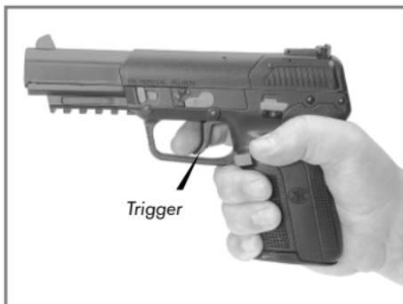
*After firing a shot, release the trigger so that it resets to the forward position.*
