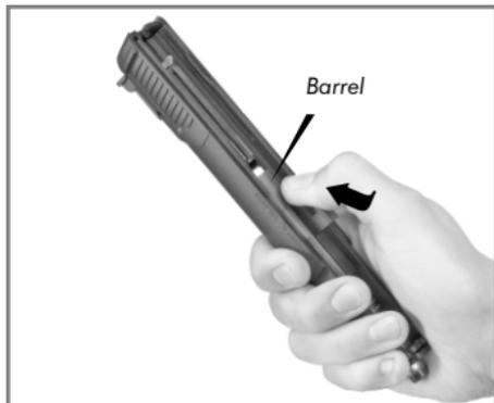
***Before carrying out the next step, ensure that the takedown lever is at the rear position, that the frame does not contain a magazine and that the hammer is in the cocked position.***
