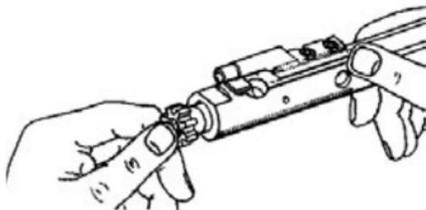
2. Remove firing pin retaining pin
