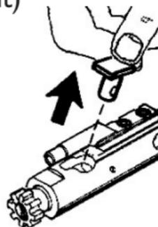
5. Remove bolt assembly from carrier.
