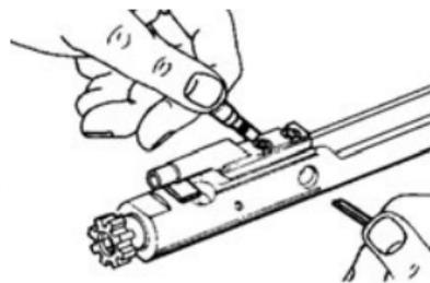
3. Drop firing pin out of rear of bolt carrier
