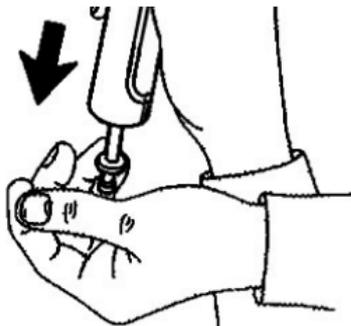
4. Remove bolt cam pin
