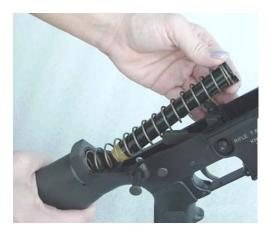
2-10 a. Depress Buffer Detent while preventing Buffer from flying-out under spring pressure with your Thumb
