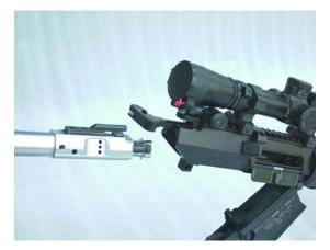
2-7 d. Withdraw Bolt Carrier Assembly
