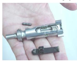
Bolt & Extractor readied for detail cleaning.
