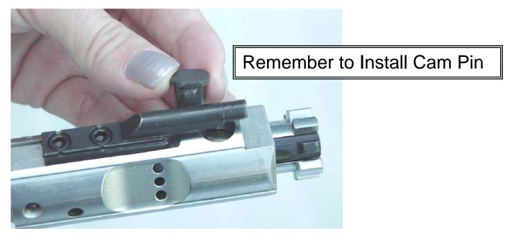
d. HOLD FIRING PIN RETAINING PIN TO ITS FULL OPEN STOP. Hold bolt downwards in palm of hand and drop firing pin into carrier. With a section of cleaning rod, push firing pin to its full forward position (only about 1/8" of the firing pin head is visible when fully forward).
