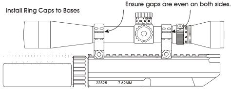
4. Install the ring caps to the bases with the screws provided with the rings. While only finger tightening the cap screws, ensure that the gap between each cap and its base is equal on both sides of the ring.
