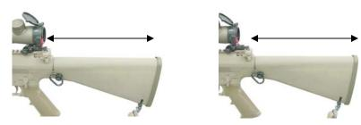
Move scope forward for eye relief with stock at shortest position.
