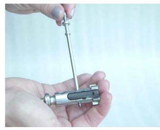
2-9 a. Push Out Extractor Pivot Pin Slightly with Firing Pin
