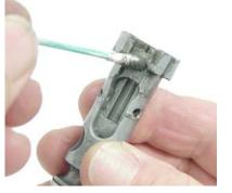
Q-Tips for Extractor & Cam Pin Recesses
