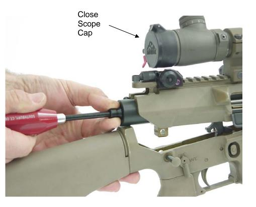
**Note:** If your cleaning patches are to large they may be to difficult to push through the bore, either cut down the patch to reduce its size, or remove the bore rod tip or jag from the rod and try just the rod end to push patches though.
