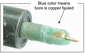
(2) Wait 5 to 10 minutes for the de-fouling chemical to attack the copper.
