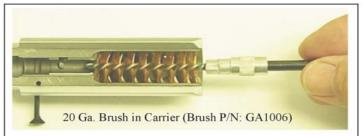
(1) Assemble the #9 Small Brass Bolt Carrier Brush to the #6 Chamber & Brass Brush Rod and insert it through the small diameter hole inside the bolt carrier. One or two passes with the brush will generally clean carbon from the bolt's tail piece recess. Rotate rod handle clockwise to keep the brush from unscrewing.
