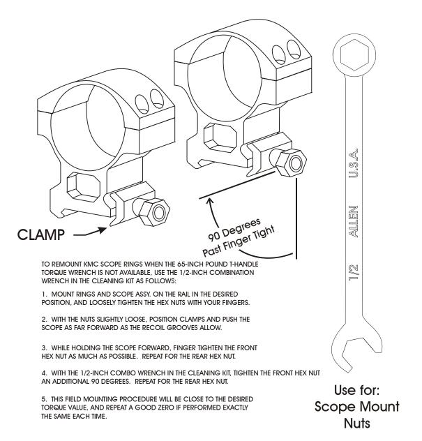
Figure B-1 Use of <sup>1</sup>/<sub>2</sub>" Combination Wrench with Scope Ring Nuts (Same for SR-M110 1-Piece Mount)
