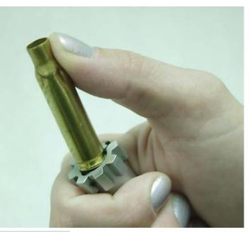
2. Hook case under extractor lip and depress ejector with thumb pressure several times.
