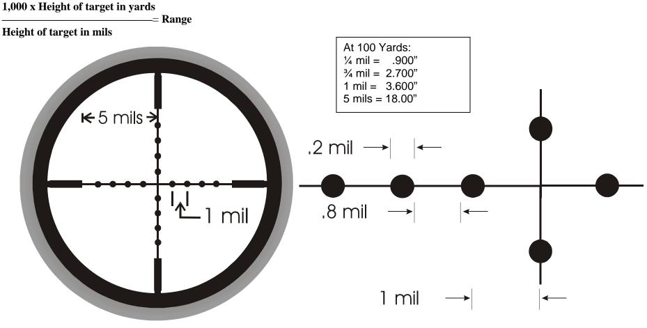
Figure 2-11 Mk 11 Mod 0 .8 Mil-Dot Reticle
