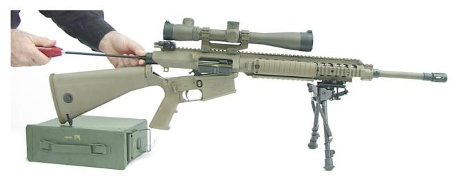
Using the Bore Rod Guide in this manner helps keep the sights up, and if the buttstock is raised as shown above, then bore solvent drains away from the chamber, while keeping the rifle stable for bore cleaning.
