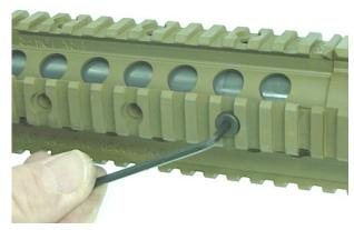
3. Remove screws form both sides.(Note: as many as 6 screws may be present.
