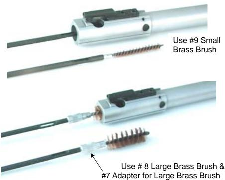
(2) Assemble the #8 Large Brass Bolt Carrier Brush and its #7 Adapter to the #6 Chamber & Brass Brush Rod and insert it in the bolt carrier's bolt recess. Rotate rod handle clockwise 5 or 6 times to keep the brush from unscrewing and to clean carbon from the bolt recess.
