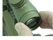
(5) Repeat Steps 2-4 until focus is set for your eyes. Mk 11: then screw the lock ring up against the eyepiece--hold the eyepiece in one hand and do not let it move as you rotate the lock ring. Turn the lock ring until finger tight against the eyepiece. **M-110 has no lock ring, it has an eyepiece diopter (focus) adjustment ring at the rear of the scope that is marked for your reference.**
