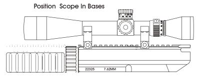
2. Remove Ring Caps and clean away any oil or dirt from the scope and ring mating surfaces. Position scope in bases as shown.
