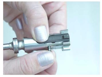
2-9 b. Withdraw Extractor Pivot Pin and Remove Extractor
