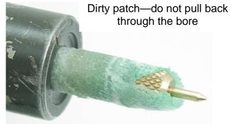
Once patches wet with bore cleaner clear the muzzle and are reasonably clean, then scrub the bore with the brass bore brush. After 5 full in-and-out strokes with the bore brush, change back to wet bore patches as described previously.
