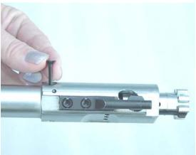
2-8 b. Pull Firing Pin Retainer Pin
