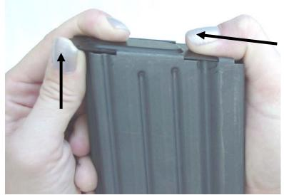
Figure 2-5b Removing Magazine Base
