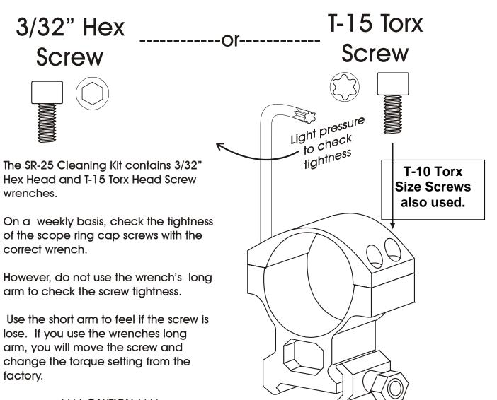
\*\*\*\* CAUTION \*\*\*\* Using the wrench's long arm may overtighten and break the screws.
