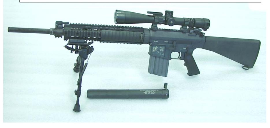
Figure 1-1 (Basic Mk 11 Mod 0 Rifle & Sound Suppressor)
