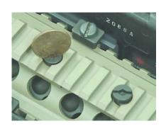
Note: Newer Screws are also slotted for turning with a coin.
