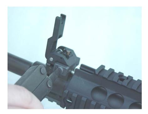
Figure 2-6 Installation of Mk 11Back-Up Front Sight
