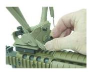
3. Tighten Bipod Pivot Tension.
