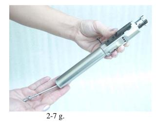
Tilt Bolt Up and Catch Firing Pin in Hand
