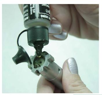
1. Apply 1 drop of CLP to the area around the ejector.
