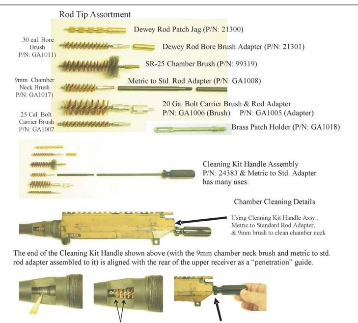
Handle Front Edge used as 9mm brush penetration limit indicator—do not push it in any further
