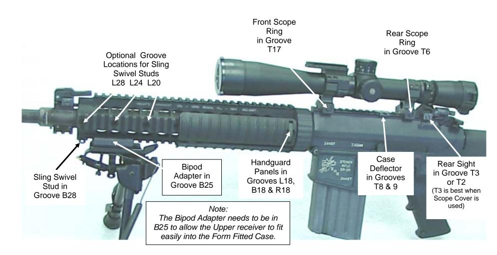
Figure 2-13 Recommended Accessory Groove Locations (Mk 11 Mod 0)
