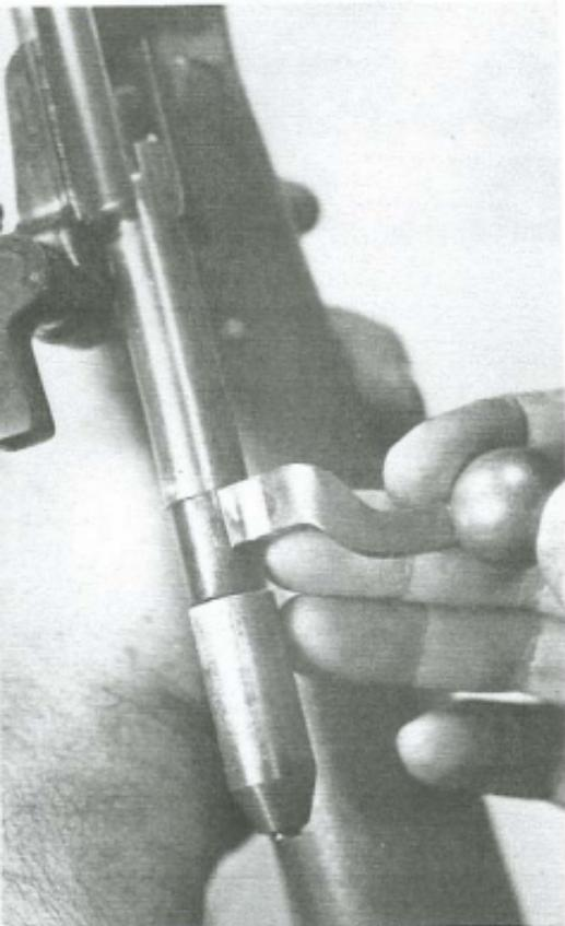
2. Turn the bolt handle clockwise (rear view) to allow the striker to move forward to the fired position.
