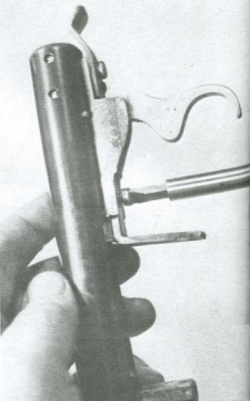
10. Remove the screw at the rear of the trigger bracket. This screw also is the pivot for the safety lever.
