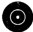
FIGURE 7 SIGHT PICTURES (what to look for when you look through the rear sight)
